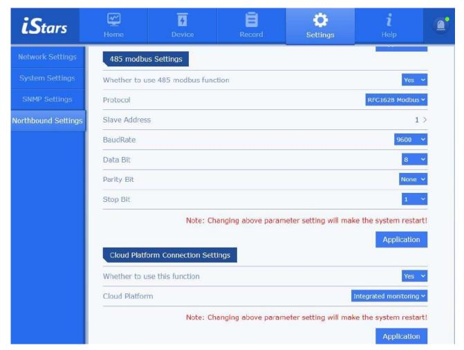
Figure 3.22 485 modbus settings, cloud platform connection settings
