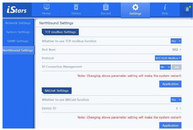
Figure 3.21 TCP modbus settings, BACnet settings
