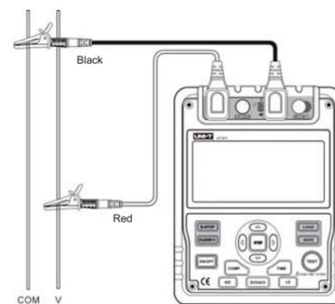
Figure 4. Voltage Measurement
