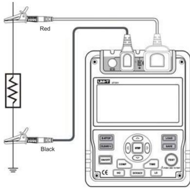
Figure 5. Insulation Resistance Measurement
