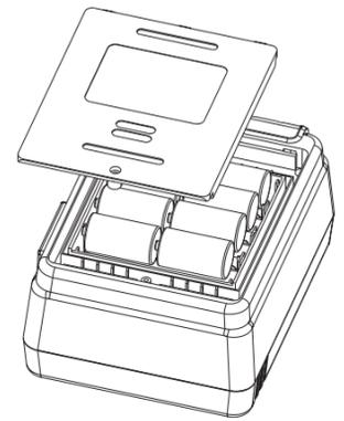
Figure 8. Battery Replacement
